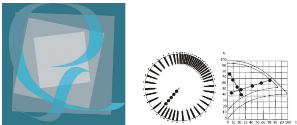
FIG. 8. A monochrome, cold blue (A55.39) composition consisting of nine colors. The colors of the composition form two scales running approximately perpendicular to each other. The colors of the first scale have a uniformly decreasing Coloroid saturation and Coloroid brightness. The colors of the other scale have a decreasing Coloroid saturation and increasing brightness.
